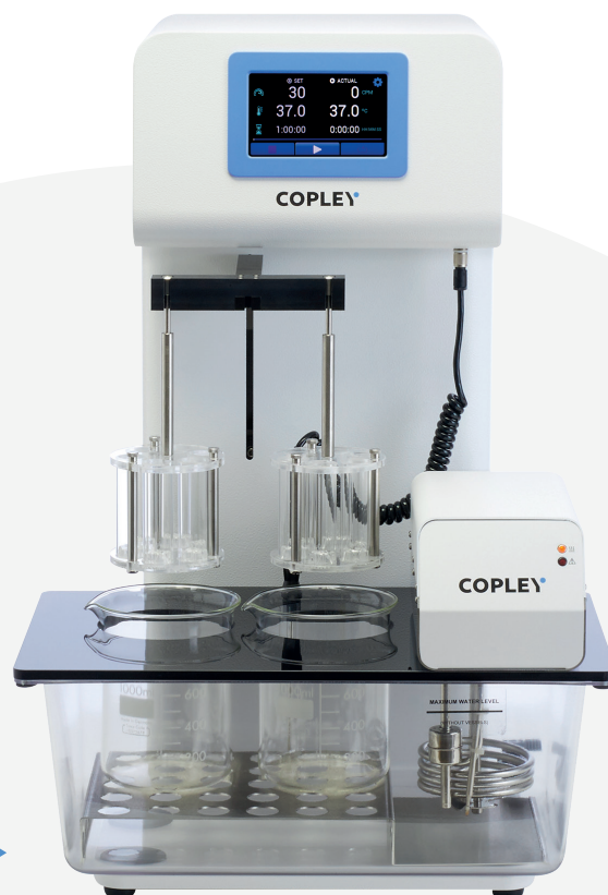
Figure 2: A simple apparatus for standardised, reproducible disintegration testing
