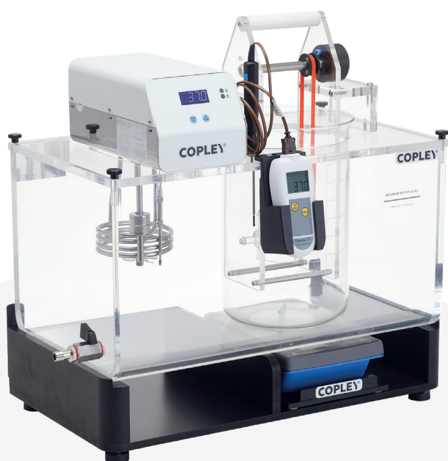
Figure 6: Disintegration testing apparatus for hydrophilic suppositories can also be used to measure the softening times of lipophilic products.
