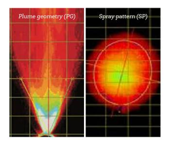
Images acquired through real time, high speed camera footage of aerosols or sprays emitted from a device allow for subsequent data analysis of spray pattern and plume geometry to determine the shape and size of the aerosol or spray.
