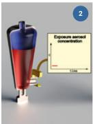
The aerosol rises upwards in a plume, then settling downwards in the holding chamber where a controlled air flow "pulls" the API past a real-time aerosol monitor.
