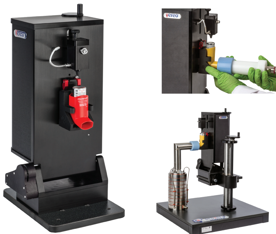
Figure 3. Proveris Vereo® SFMDx actuator for pMDI products (left); SFMDx with DCU setup (top right) and Anderson Cascade Impactor (bottom right).
