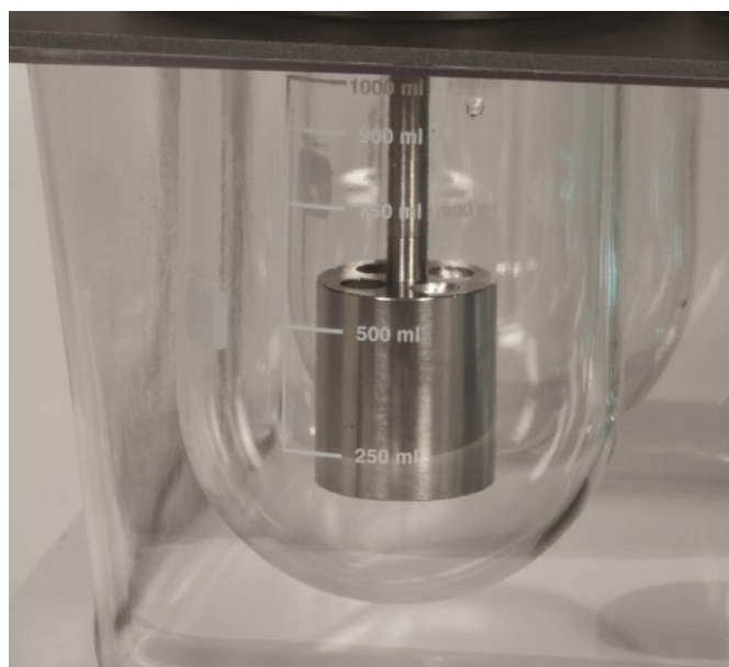
Figure 5: Methods for performance testing for TDPs use modified OSD dissolution testing apparatus and include: Rotating Cylinder (left) and Paddle over Disk (right).
