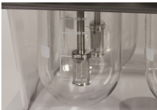
Figure 3: The most common types of dissolution testing apparatus are Apparatus 1 (Basket) and Apparatus 2 (Paddle)
