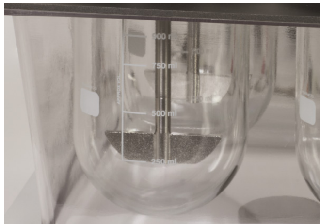
Figure 3: The most common types of dissolution testing apparatus are Apparatus 1 (Basket) and Apparatus 2 (Paddle)
