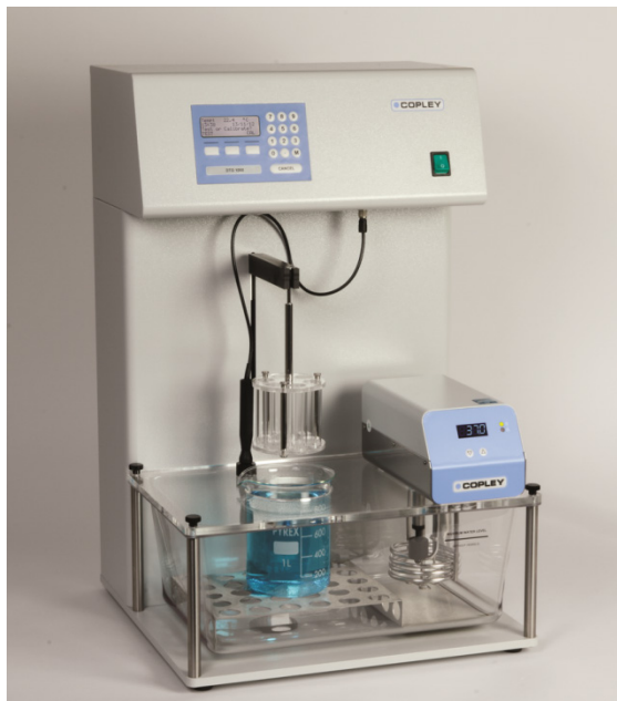
Figure 2: A simple apparatus for standardised, reproducible disintegration testing
