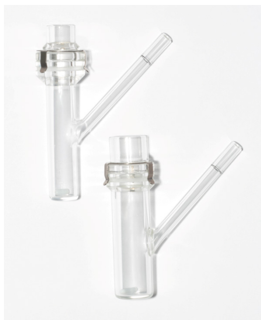
Figure 4: 7 and 20 ml VDC designs are available for testing different volumes of semisolids.
