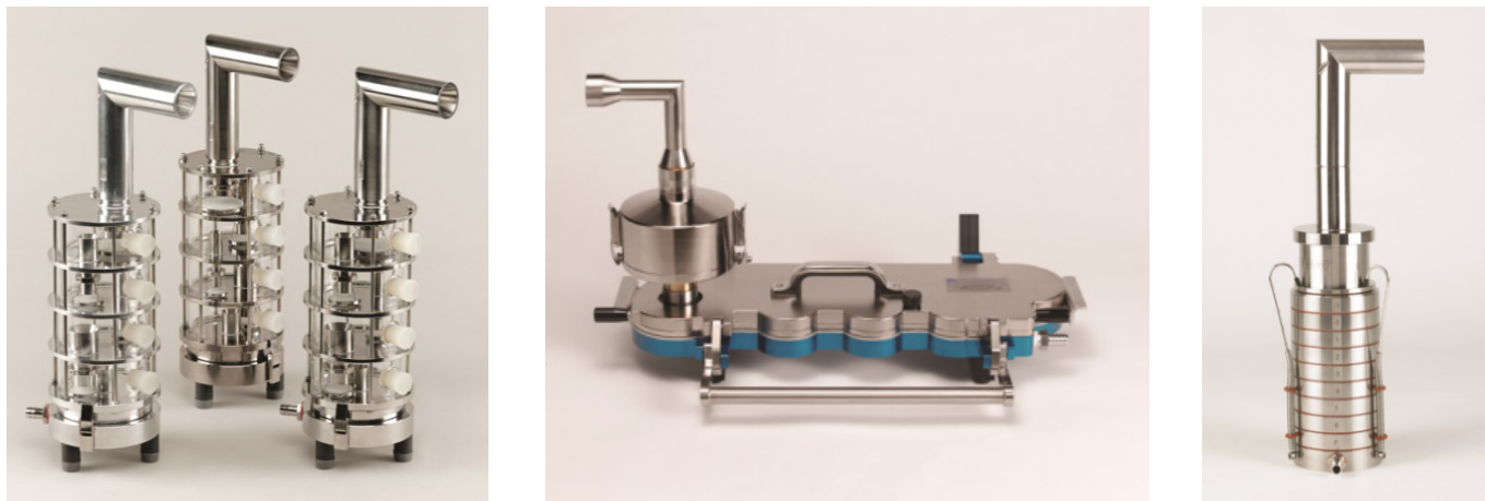
Figure 8: The MSLI, NGI and ACI are all referenced in compendial methods for determining the APSD of OIPs but the NGI and ACI are the instruments of choice for the majority of testing.
